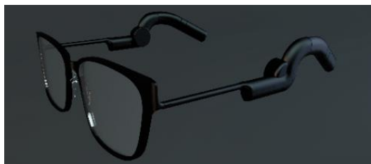
"Spectacle Hearing Device" (prototype) equipped with bone-conduction speakers and a microphone, currently under development by freecle Inc.
